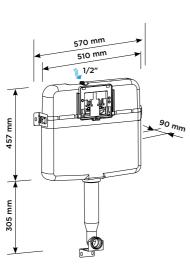
Product Code: TC200CONC Notes: Flush-plate sold separately. 6 litres insulated cistern, conforms to EN 14055 class 2 flushing standard. Dual flush valve factory set to 6/4 litres, adjustable to 4.5/3 litres on site, if required.
