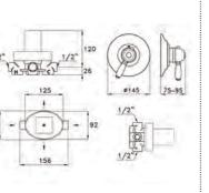
Notes: This thermostatic shower has two outlets, which can be used for the control of one or two water supplies, ONLY when combined with ADDITIONAL stop valves (e.g. TCSH19209154).
